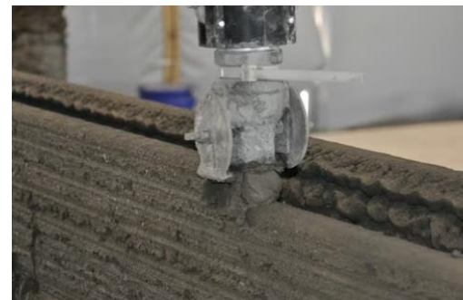
U.S. Army Engineer Research and Development Center, Construction Engineer Research Laboratory's concrete 3D printing apparatus. US Army. 2020.
